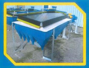
Table tilt can be easily adjusted using a hand wheel, even while the machine is in operation. Iolman-Willi
