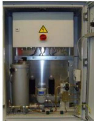
Figure: Exemplary Central Grease Lubrication unit
