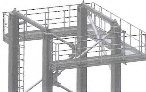
Lift the CT33 – using the temporary lifting yokes on top of the CT33 – and fit the CT33 on the supports on B33.
